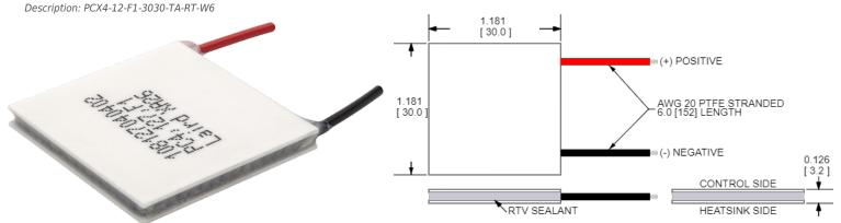
CERAMIC MATERIAL: Al₂O₃ SOLDER CONSTRUCTION: 232°C, SbSn
