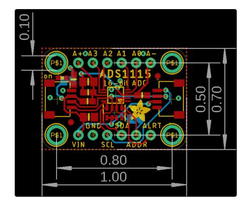
Schematic and Fab Print Original Version (Identical For Both)
