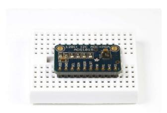
Position the breakout board Place the breakout board on the header pins.
