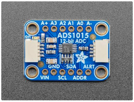
The ADS1115 and ADS1015 4-channel breakout boards are perfect for adding high-resolution analog to digital conversion to any microprocessor-based project. These boards can run with power and logic signals between 2v to 5v, so they are compatible with all common 3.3v and 5v processors. As many of 4 of these boards can be controlled from the same 2-wire I2C bus, giving you up to 16 single-ended or 8 differential channels. A programmable gain amplifier provides up to x16 gain for small signals.
