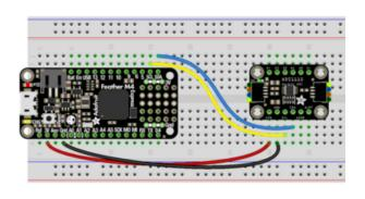
Board 3V (red wire in STEMMA QT version) to ADS1x15 VDD - Remember the maximum input voltage to any ADC channel cannot exceed this VDD 3V value! Board GND (black wire in STEMMA QT version) to ADS1x15 GND Board SCL (yellow wire in STEMMA QT version) to ADS1x15 SCL Board SDA (blue wire in STEMMA QT version) to ADS1x15 SDA
