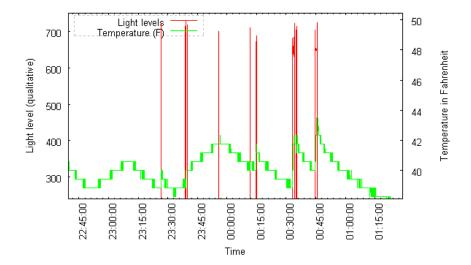
Zooming into the plot at about 12:40AM, we can see how the temperature climbs whenever the door is open, even in a few seconds it can climb 4 degrees very quickly!
