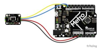
Connect Vin to the power supply, 3-5V is fine. (red wire on STEMMA QT version)
