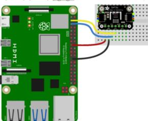
Pi 3V3 to sensor VIN (red wire on STEMMA QT version) Pi GND to sensor GND (black wire on STEMMA QT version) Pi SCL to sensor SCL (yellow wire on STEMMA QT version) Pi SDA to sensor SDA (blue wire on STEMMA QT version)
