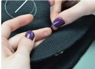
You can start with the pixel + or -. For this hat we chose to start with the shared ground line that hooks up all the sequins. Stitch around the GND pad on GEMMA at the edge of a knit cap and knot/seal at the back.
