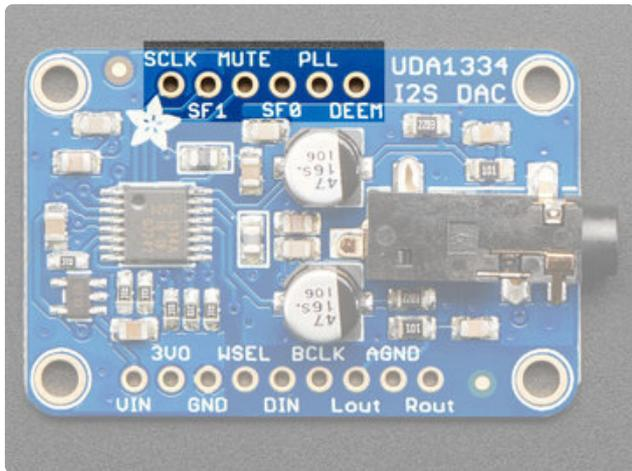
**SCLK (Sys Clock)** - Optional 27 MHz 'video mode' system clock input - by default we generate the sysclock from the WS clock in 'audio mode' But the UDA can also take an oscillator input on this pin
