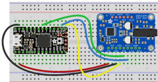
Connect **VIN** on the breakout to **3V/3.3** on the board.
