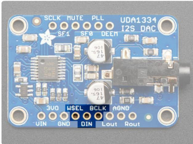
**WSEL** (Word Select or Left/Right Clock) - this is the pin that tells the DAC when the data is for the left channel and when its for the right channel
