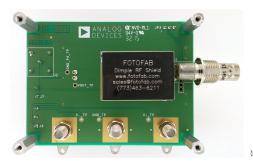
Figure 22. Evaluation Board Bottom View with SHIELD3
