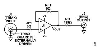
Figure 6. Buffer with Triax Guard Externally Driven Schematic
