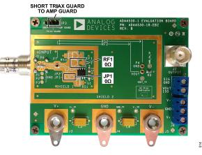
Figure 7. Buffer with Triax Guard Driven by Amp Guard
