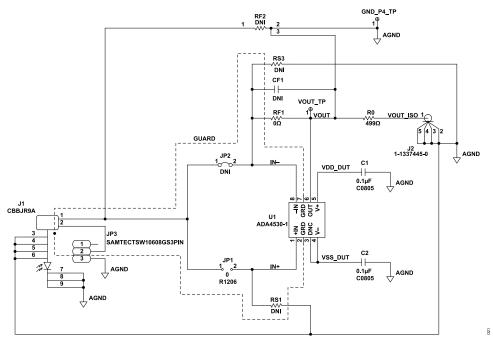
Figure 25. ADA4530-1R-EBZ-BUF Schematic
