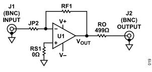
Figure 20. Inverting Gain Schematic
