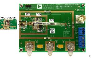
Figure 17. Transimpedance with Direct Sensor Connection
