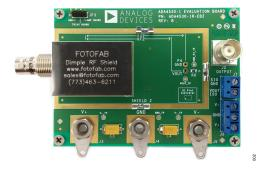
Figure 21. Evaluation Board Top View with SHIELD1
