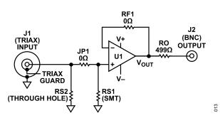
Figure 10. Buffer with Resistor at IN+ to Ground Schematic
