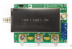
Figure 23. Evaluation Board Top View with SHIELD2
