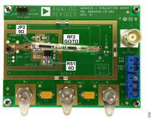
Figure 15. Transimpedance with Through Hole Feedback Resistor
