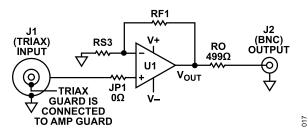
Figure 12. Noninverting Gain Schematic
