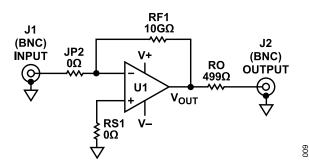
Figure 14. Transimpedance with 10 G $\Omega$  Feedback and IN+ Connected to Ground Schematic
