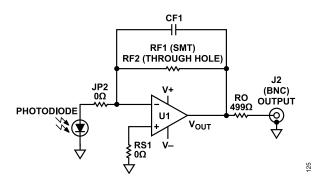
Figure 18. Transimpedance with Direct Sensor Connection Schematic
