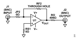
Figure 16. Transimpedance with Through Hole Feedback Resistor Schematic
