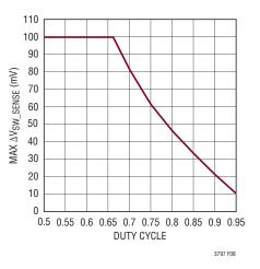
Figure 8. The Maximum Sense Voltage Ripple vs Duty Cycle for CCM
