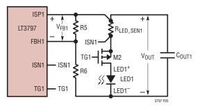
Figure 3. Output Voltage Sense Resistor Connection
