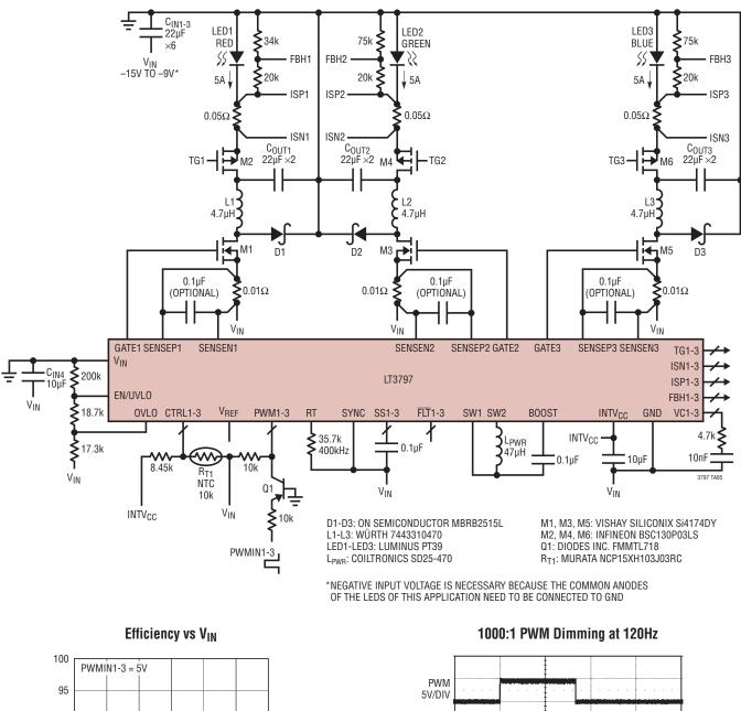
Triple Buck Mode LED Driver for Common Anode LEDs
