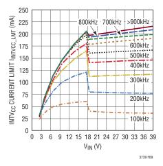
Figure 9. INTV<sub>CC</sub> Current Limit vs  $V_{IN}$ ,  $f_{SW}$
