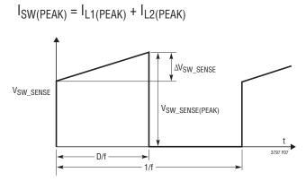
Figure 7. The Sense Voltage Across the Sense Resistor in CCM
