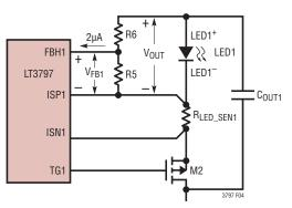
Figure 4. Output Voltage Sense Resistor Connection When R<sub>LED SEN1</sub> and M2 Are Connected to the Bottom of the LED String
