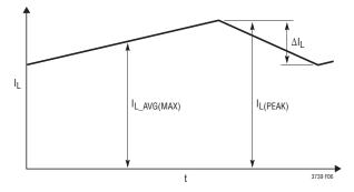
Figure 6. A Typical Inductor Waveform
