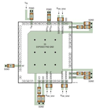
Figure 10. Decoupling Capacitors and Ground Separation
