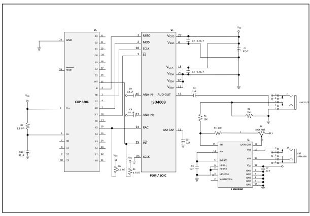
FIGURE 11: APPLICATION EXAMPLE USING SPI PORT ON MICROCONTROLLER
