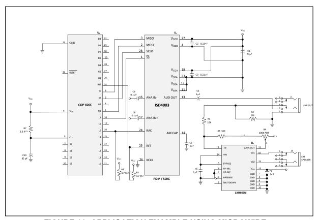
FIGURE 10: APPLICATION EXAMPLE USING MICROWIRE
