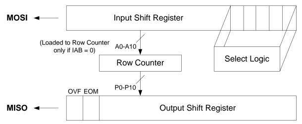
FIGURE 3: SPI INTERFACE SIMPLIFIED BLOCK DIAGRAM
