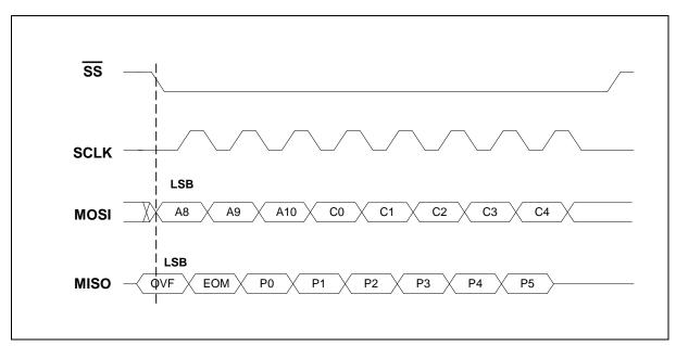
**FIGURE 6: 8-BIT COMMAND FORMAT**
