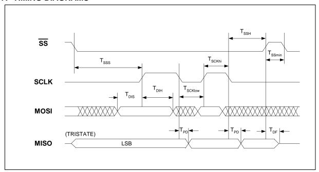
**FIGURE 5: TIMING DIAGRAM**
