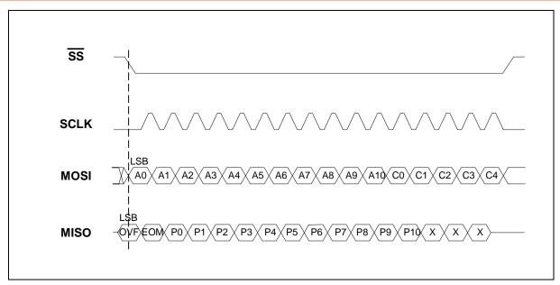
**FIGURE 7: 16-BIT COMMAND FORMAT**
