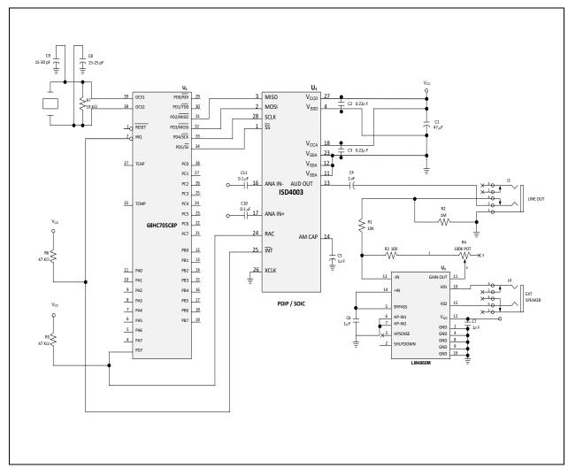
FIGURE 9: APPLICATION EXAMPLE USING SPI
