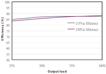
Fig. 1 Efficiency versus output load
