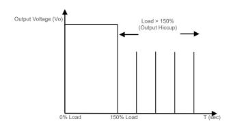
Additionally, if the  $I_0$  is <210% but >150% for a prolong period of time (depending on the load), the Over Temperature Protection (OTP) will be activated due to high temperature on critical components. The power supply will then go into hiccup mode until the fault is removed; and, the input voltage is removed, then reapplied.
