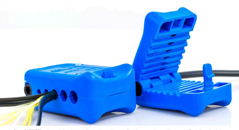
These **PATENTED** tools are designed to open fiber jackets and loose buffer tubes to provide easy fiber access. The buffer tube slitting is done without damage to the fiber. Blades are replaceable.
