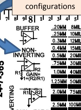
The trace width examples were made with both MIL & MM on both sides for ease of comparison between the two.
