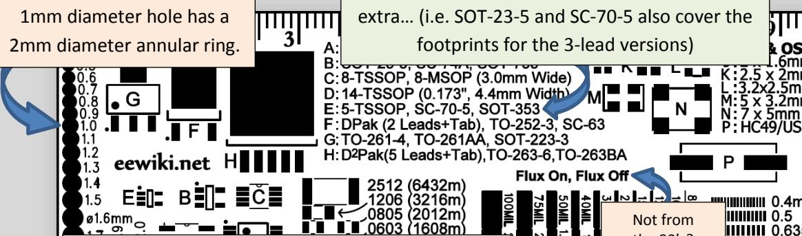
The trace width examples, on this side, were positioned on the edge so they could be placed over a PCB trace to estimate what width was used.
