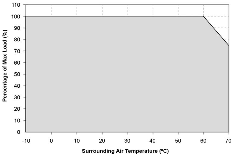
**Fig. 1 De-rating for Vertical and Horizontal Mounting Orientation**
