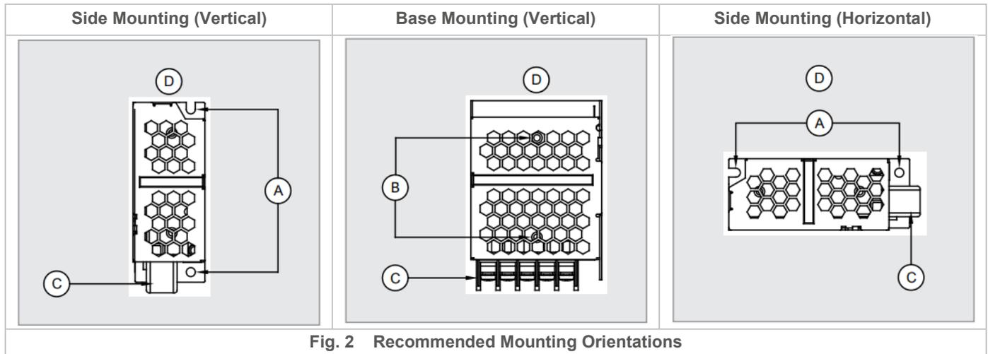
Fig. 2 Recommended Mounting Orientations
